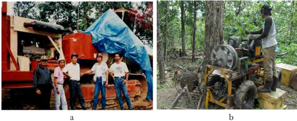
Figure 10. Sophisticated skyline machine of TTY 70 (a) and a simple prototype G-3 (b)
