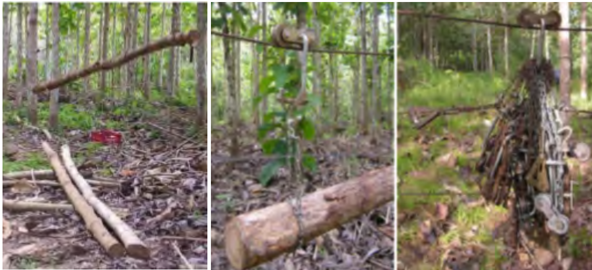
Figure 9. Logs extracted using simple hoist made by small pulleys and nylon string loading -unloading.
